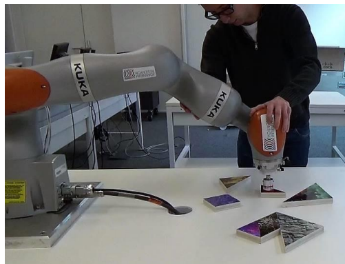
Figure 1. A collaborative robot (KUKA iiwa 4 ) working together with a human. 5
