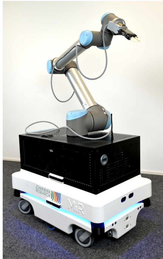
Fig. 1. The CHIMERA mobile manipulator in its default configuration with UR10 arm and MiR100 mobile base.
