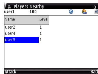
Figure 3. A screenshot of Geobashing showing the players in range. The three icons at the top right indicate (left to right) that GPS is online, players are in range and that the player is logged in.
